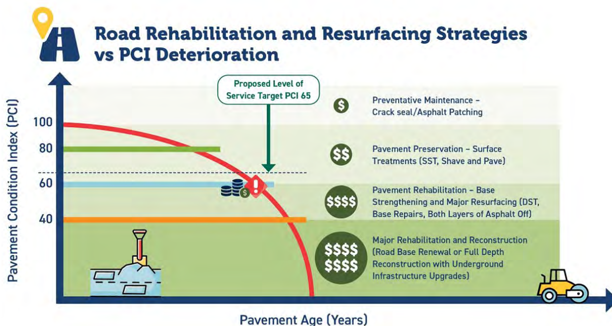
Figure 1: Road Rehabilitation and Resurfacing Strategies vs PCI Deterioration
