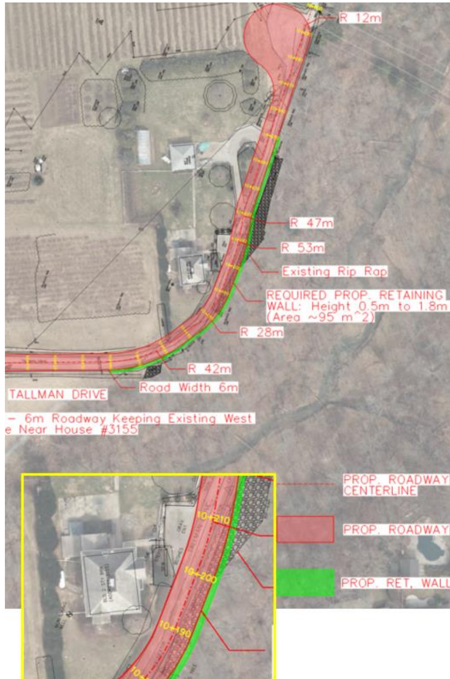
Figure 5-1 Solution #1 - Reconstruct / Rehabilitate Existing Road
