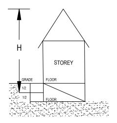
WHEN 'A' IS GREATER THAN 'B' THAN 'C' IS BASEMENT WHEN 'A' IS LESS THAN 'B' THEN 'C' IS A CELLAR
